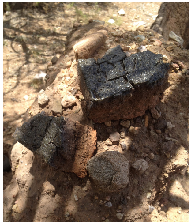
Figure 4. Adobes which were part of the smelter wall were exposed to such high heat that portions turned to glass (photo by Dan Judkins, 2015).
